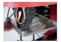
Manual Tooling J-Frame is used for small boxes and short reverse flanges
